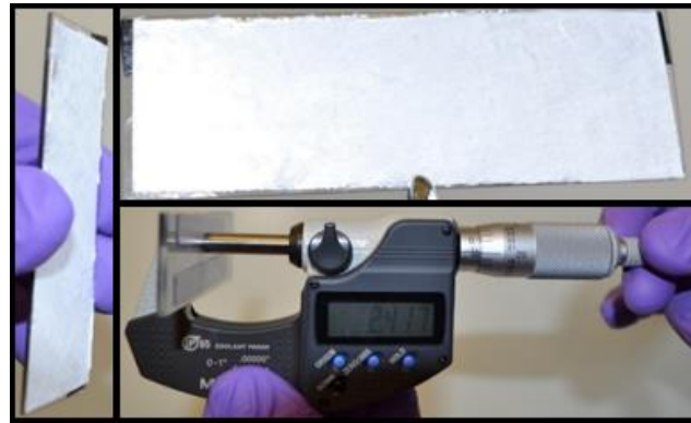
Figure 3.2: Using Micrometer to Measure the Thickness.
